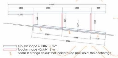
Anchored to the beams (Z shape, IPE, C...) the truss presents a perfect distribution of loads, so it leans perpendicularly on each and every of the beams, in addition it does not involve any overload for the roof because it is made up by tubular shape with a thin thickness that affects load lower than **5 kg / m2**
